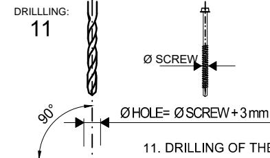
11. DRILLING OF THE SHEETS CAN BE EXECUTED ON SITE BY MEANS OF A DRILL AND SUITABLE HEADS. THE HOLE MUST BE 3mm WIDER THAN SCREW GAUGE OR A SLOT ALONG THE LENGTH
