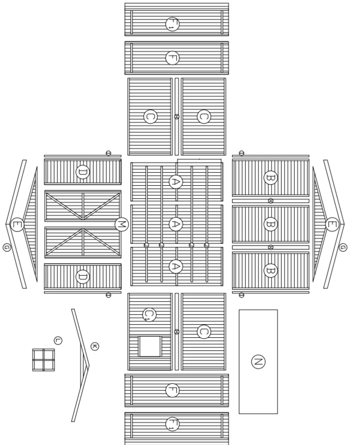
1. place 4 elements ( J ) under 3 floor elements ( A ) and fasten each element with 4 x 30 mm screws as shown in the picture
