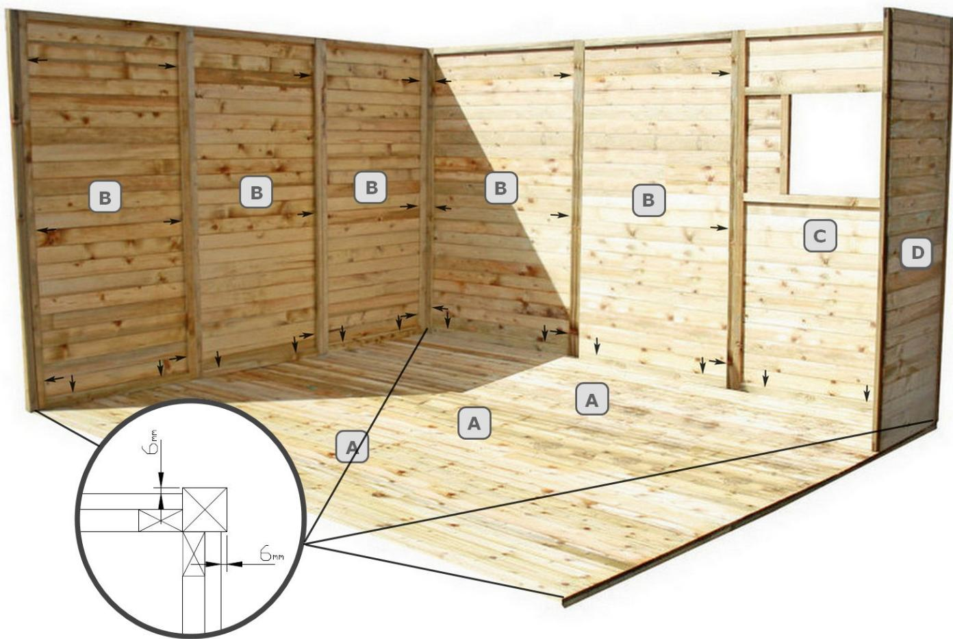
3. all walls should be assembled as described in point 2 with 4.5 x 70 screws
